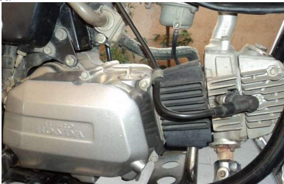
Figure 3: Four Stroke Single Cylinder Petrol Engine
